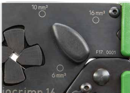
Only for "Variocrimp 16": Adjust conductor cross section with crimping tool in open position.
