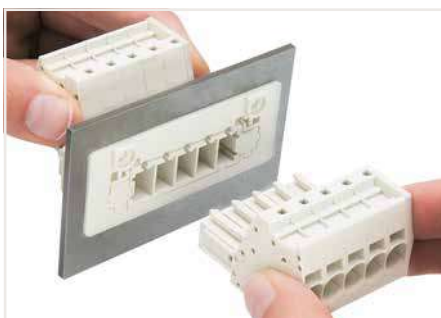
Inserting a female connector without lateral locking levers – lockout pins are inserted on both sides of the snap-in frame.
