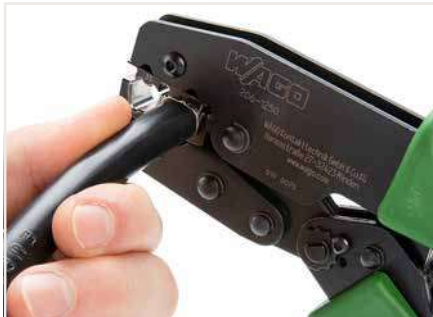
Squeeze handles until ratchet mechanism is released.
