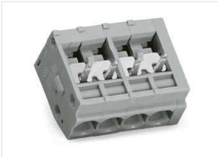
WAGO's 805 Series Terminal Strips provide "internal commoning" to meet requirements that ban routing the ground conductor over the board. This enables custom terminal strips to be commoned and marked at the factory upon request.
