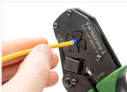
Squeeze handles until ratchet mechanism is released.
