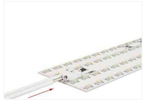
Insert solid conductors via push-in termination.
