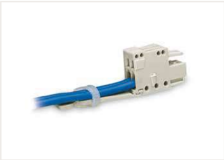
Strain relief plate; for factory assembly; 1-conductor female connector; 2.5 mm pin spacing; light gray; 2-pole, with strain relief plate (733-102/032-000)
