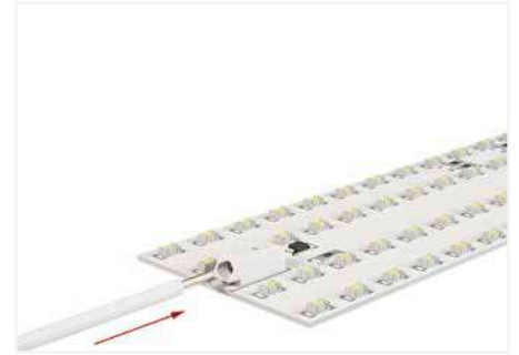
Insert solid conductors via push-in termination.
