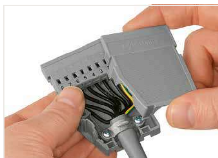
Snapping on a strain relief housing, demonstrated with a female connector with locking levers. Cable exits laterally – strain relief by cable tie (up to a width of 4 mm).
