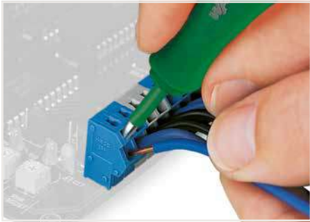
Removing a conductor.
