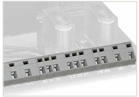
Combining PCB terminal blocks with different pin spacing.
