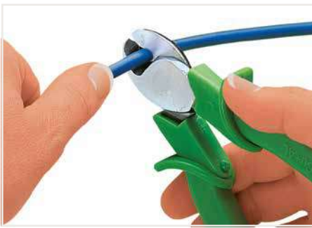
Cutting a cable.
