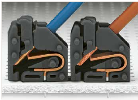
Inserting solid conductors via push-in termination. Inserting fine-stranded conductors via push-buttons, 250 Series – 3.5 mm pin spacing.
