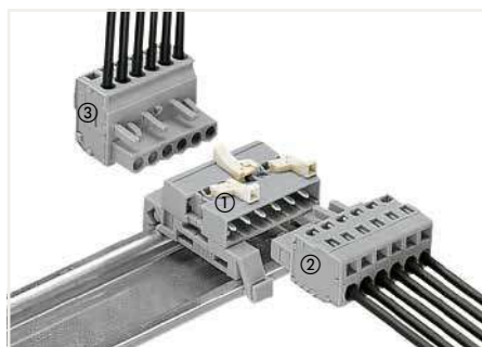
① Double-pin male connector with mounting feet, for DIN-35 rail ② Female connector with CAGE CLAMP® ③ Angled female connector with CAGE CLAMP®, conductor exit same direction as latches
