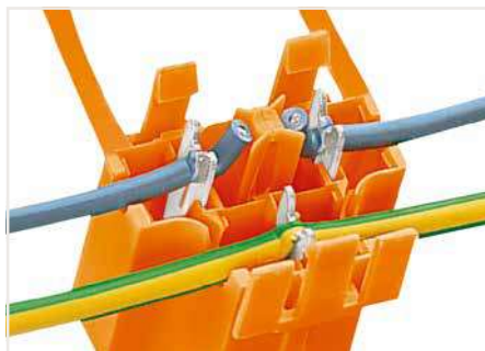
Snapping socket halves together will automatically cut and terminate a "live" conductor without stripping – enables switching applications (e.g., door switches).
