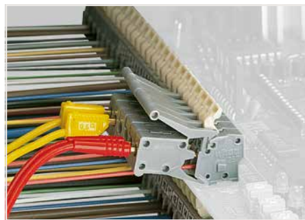
Testing with test plug modules.
