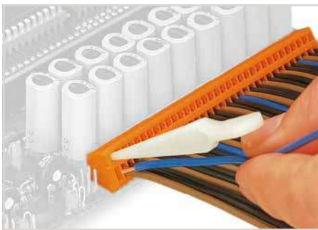
Inserting a conductor via 233-332 Operating Tool. Operation is performed parallel to conductor entry.
