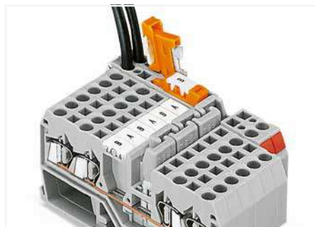
Staggered jumpers for sophisticated circuit requirements – push jumpers down until fully inserted.
