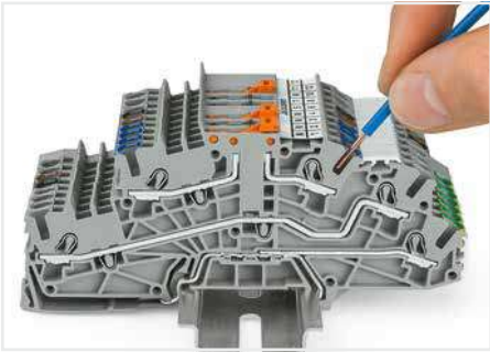
Inserting a conductor via push-in termination. Solid conductors with cross-sections from either one size above, or up to two sizes below, the rated cross-section can be simply pushed in – no tools needed.
