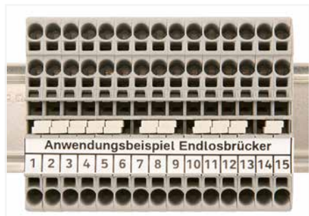
Continuous jumpers (2002 Series) readily connect an endless number of terminal blocks to each other via single jumper slot. Use the second jumper slot for additional commoning or testing.
