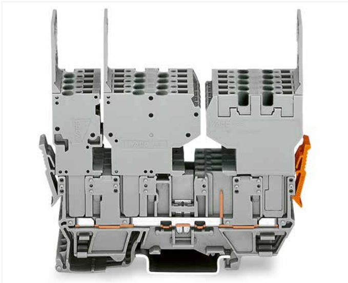
1-conductor and 2-conductor female plugs (left), 2-conductor female plug (right), may be reversed – carrier terminal blocks can only be commoned via 280 Series Adjacent and Alternate Jumpers.
