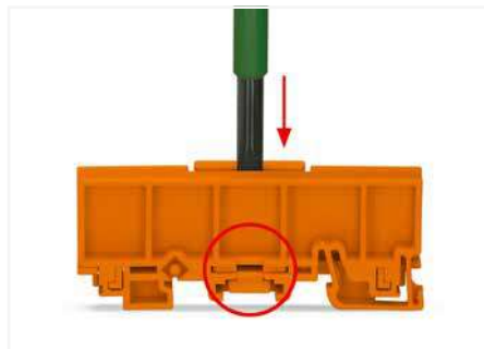
One single carrier can hold up to 24 clamping units in a very narrow space. Previously, this was only possible using rail-mount terminal blocks.
