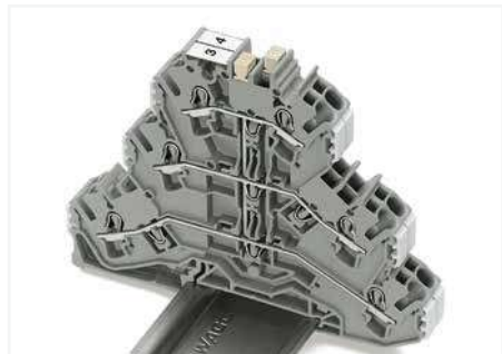
Commoning three levels via triple-deck vertical jumper (2002-493).
