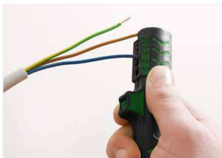
Stripping a conductor insulation.
