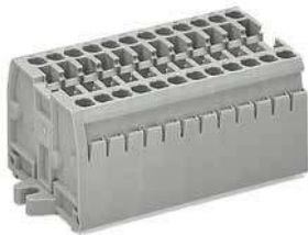
Compact terminal strip; with M3 mounting flanges; for screw or similar mounting types; 3.2 mm mounting hole diameter; gray
