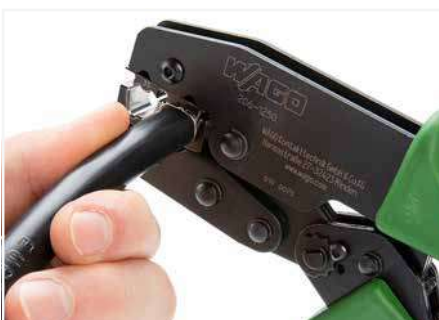
Squeeze handles until ratchet mechanism is released.
