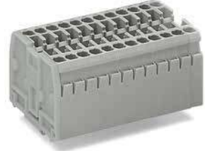
Compact terminal strip; with snap-in mounting feet; for 0.6 ... 1.2 mm plate thickness; 3.5 + 0.1 mm mounting hole diameter; gray
