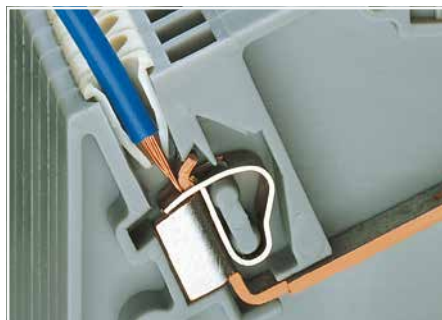
Insulation stop: Prevents the conductor insulation from being pushed into the clamping unit. (Available for terminal blocks up to 4 mm²/12 AWG)
