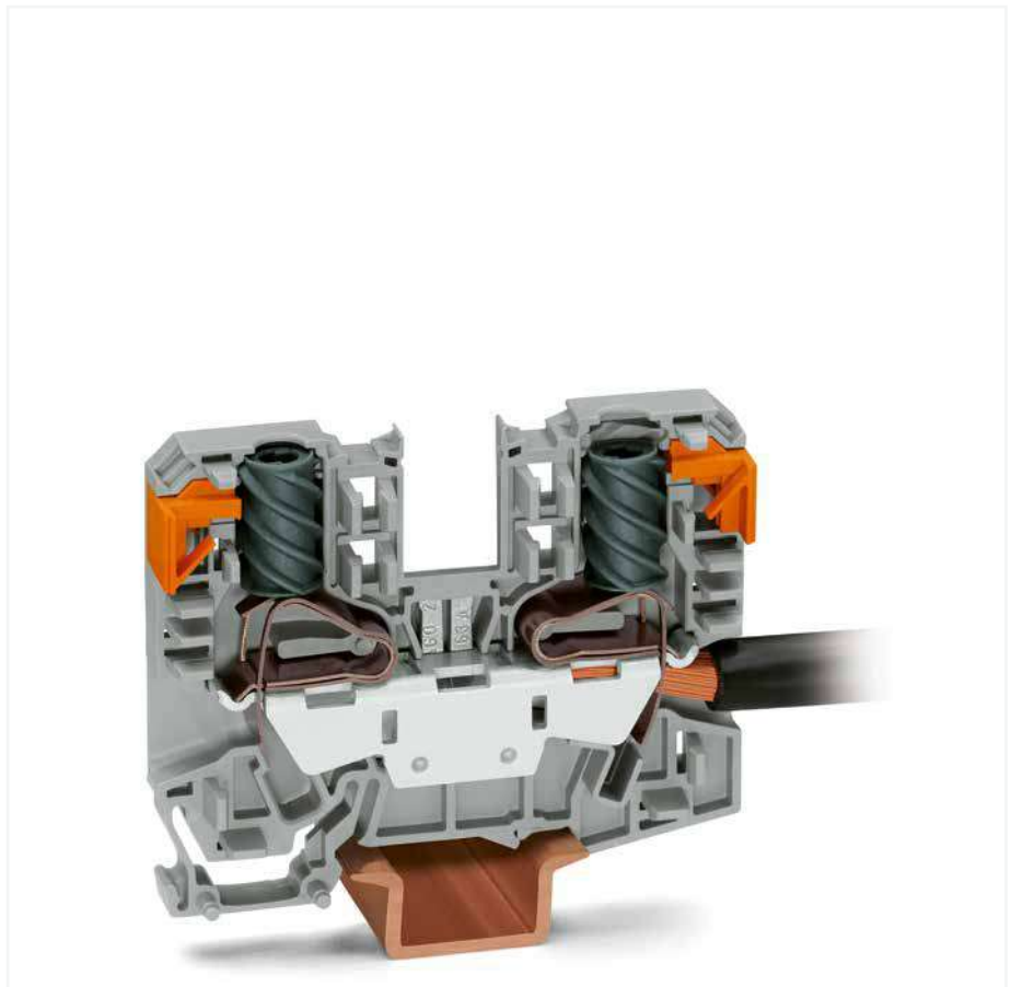
Conductor termination – step 3: A short counter-clockwise rotation closes the clamp, securing the conductor ①. When unlocked, allow operating tool to rotate clockwise ② to securely terminate the conductor.
