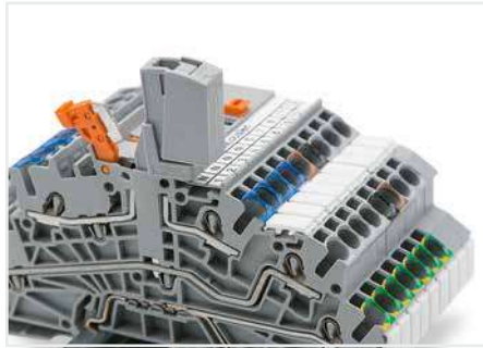
For multilevel installation terminal blocks with internal N-disconnection, test plug adapters can be inserted into the free vertical test slot when the N-potential is disconnected.
