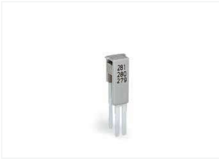
Step-down jumper from 10/6 mm 2 (8/10 AWG) to 4/2.5/1.5 mm 2 (12/14/16 AWG) I N 15 A, Item No. 284-414
