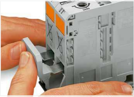
Commoning with an adjacent jumper: insert the jumper above the conductor entry hole – prior to conductor termination. The nominal cross-section remains unchanged.
