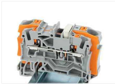
Step-down jumper (2006-499) commons 6/4 mm 2 (10/12 AWG) terminal blocks (2206/2204 Series) with 4/2.5/1.5 mm 2 (AWG 12/14/16) terminal blocks (2204/2202/2201 Series).
