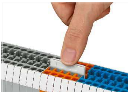
Push jumper bars down firmly until fully inserted. When using multipole bars, push alternately on the right and then left side until installed.
