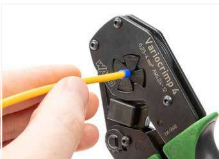
Squeeze handles until ratchet mechanism is released.
