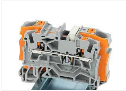
Step-down jumper (2006-499) connects 6/4 mm 2 (10/12 AWG) terminal blocks (2206/2204 Series) with 4/2.5/1.5 mm 2 (AWG 12/14/16) terminal blocks (2204/2202/2201 Series).
