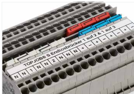
The 1-to-3 Continuous jumper enables every other terminal block to be commoned. For example, positive and negative potentials can be accommodated alongside each other.
