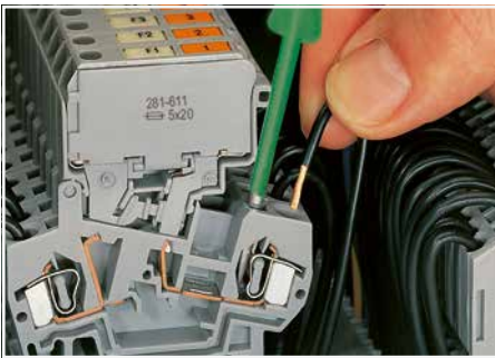
CAGE CLAMP® connection Inserting a conductor. With ferruled conductors, it is necessary to use a terminal block one size smaller than the conductor's nominal cross section.
