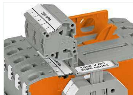
Alternatively, measurement can also be performed using Connectors (2006-511) from terminal block 1 to 2. Spacer modules (2006-549) must be used to compensate for the 15 mm terminal block width.
