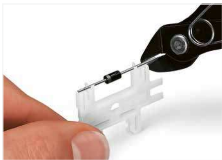
Cutting component to the proper length.
