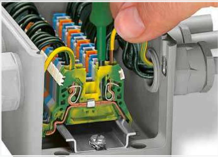
CAGE CLAMP® termination: Inserting a conductor via operating tool (0.08 ... 4 mm² "f-st"). With ferruled conductors, it is necessary to use a terminal block one size smaller than the conductor's nominal cross section.
