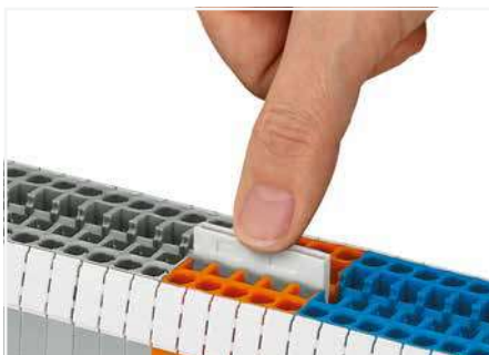
Push jumper bars down firmly until fully inserted. When using multipole bars, push alternately on the right and then left side until installed. Push-in type jumper bars 1-3-5-7 or 1-4-7 are available upon request.
