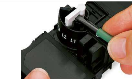
Lift jumper out of delivery position (L2) using a screwdriver and move it into the desired position.
