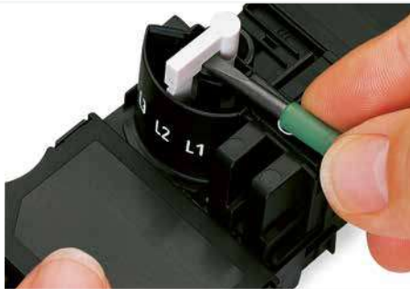
Lift jumper out of delivery position (L2) using a screwdriver and move it into the desired position.
