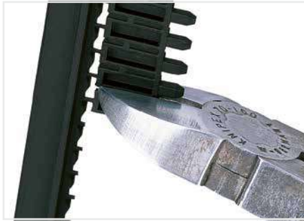
Remove unrequired areas from the sidewalls.
