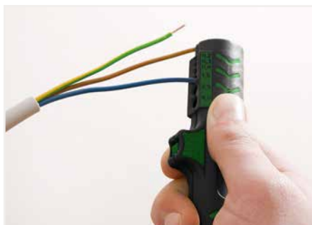
Stripping the conductor insulation.
