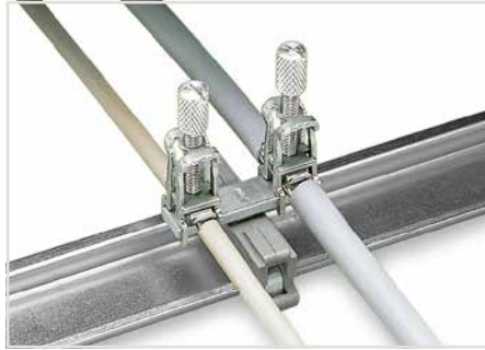
Carrier with grounding foot* (790-114), 45 mm long, busbar parallel to the DIN-rail
