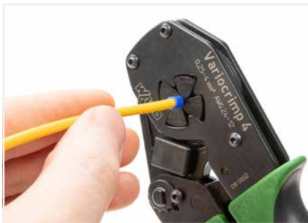
Squeeze handles until ratchet mechanism is released.
