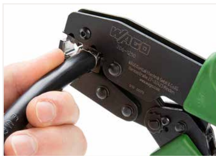
Squeeze handles until ratchet mechanism is released.
