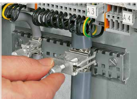
Tightening/removing a shield clamping saddle.
